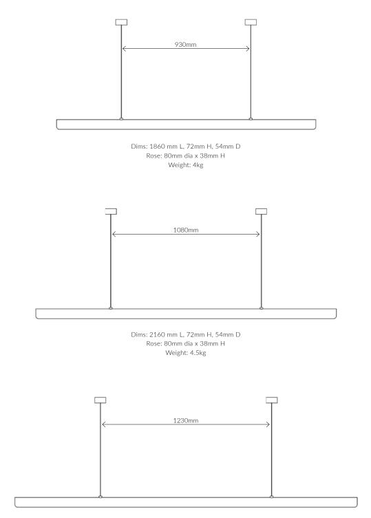
Dims: 2460 mm L, 72mm H, 54mm D Rose: 80mm dia x 38mm H Weight: 5kg
