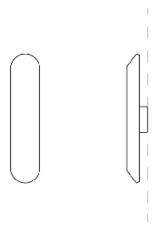
Dims: 400mm H x 90mm W x 65mm D Weight: Brass 3kg, Aluminium 1kg
