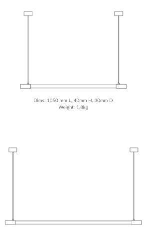
Dims: 1350 mm L, 40mm H, 30mm D Weight: 2kg
