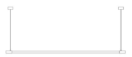
Dims: 1950 mm L, 40mm H, 30mm D Weight: 2.6kg
