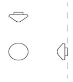
Dims: 150mm DIA x 80mm D Weight: Brass 1.8kg Aluminium 0.7kg Ceramic 1kg
