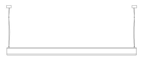
Dims: 2200 mm L, 130mm H, 75mm D Weight: 9kg
