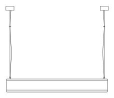
Dims: 1000 mm L, 130mm H, 75mm D Weight: 3.5kg
