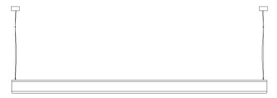
Dims: 2500 mm L, 130mm H, 75mm D Weight: 10.5kg
