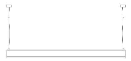
Dims: 1900 mm L, 130mm H, 75mm D Weight: 7.5kg
