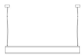
Dims: 1300 mm L, 130mm H, 75mm D Weight: 5kg
