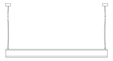
Dims: 1600 mm L, 130mm H, 75mm D Weight: 6kg
